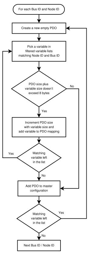
Figure 2: PDO mapping diagram
